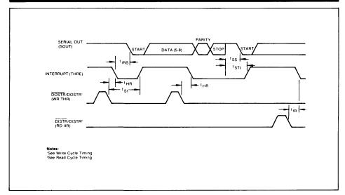
FIGURE 9. TRANSMITTER TIMING
