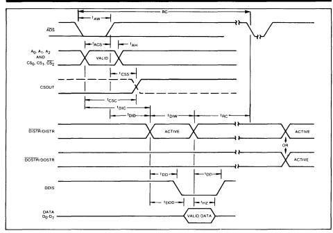
FIGURE 5. READ CYCLE TIMING
