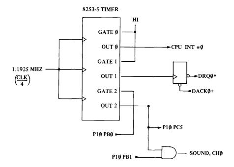
CHANNEL Ø: MODE Ø, INTERRUPT ON T/C
