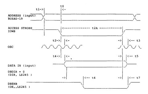
Figure 4. I/O CHIP SELECT PARAMETERS, WRITE
