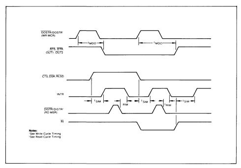
FIGURE 10. MODEM CONTROLS TIMING
