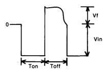
Collector Voltage Waveform
