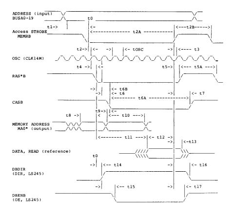
Figure 1. MEMORY TIMING PARAMETERS, READ
