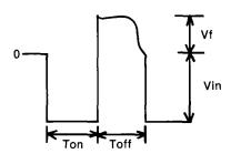
Collector Voltage Waveform
