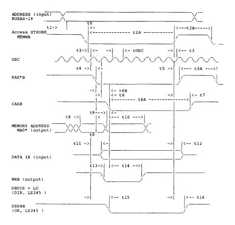
Figure 2. MEMORY TIMING PARAMETERS, WRITE
