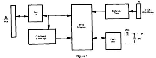
DIGI-Mouse/Clock Controller Board Block Diagram I/F
