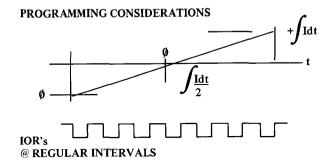
ONCE TRIGGERED BY SOFTWARE THE INTERGRATOR CIRCUIT PRODUCES A PULSE THE DURATION OF WHICH IS DEPENDENT ON JOYSK POSITION.
