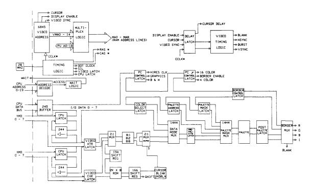
Figure 14 Video Controller Block Diagram
