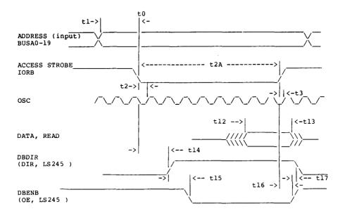
Figure 3. I/O CHIP SELECT PARAMETERS, READ
