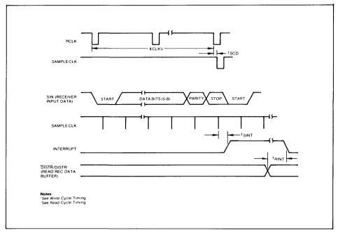
FIGURE 8. RECEIVER TIMING
