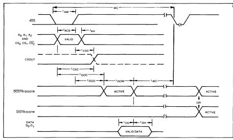
FIGURE 6. WRITE CYCLE TIMING
