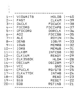
Figure 1. Pin Assignment
