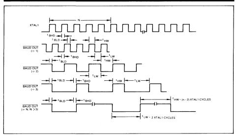
FIGURE 7. BAUDOUT TIMING
